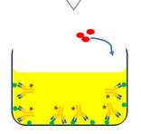
3. Add 50  $\mu$ L Stop Solution to each well, shake plate on a plate shaker for 1 minute to mix. Record the OD at 450 nm immediately, calculation of the results.
