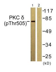
Western blot analysis of lysates from NIH/3T3 cells treated with UV 15', using PKC delta (Phospho-Thr505) Antibody. The lane on the right is blocked with the phospho peptide.
